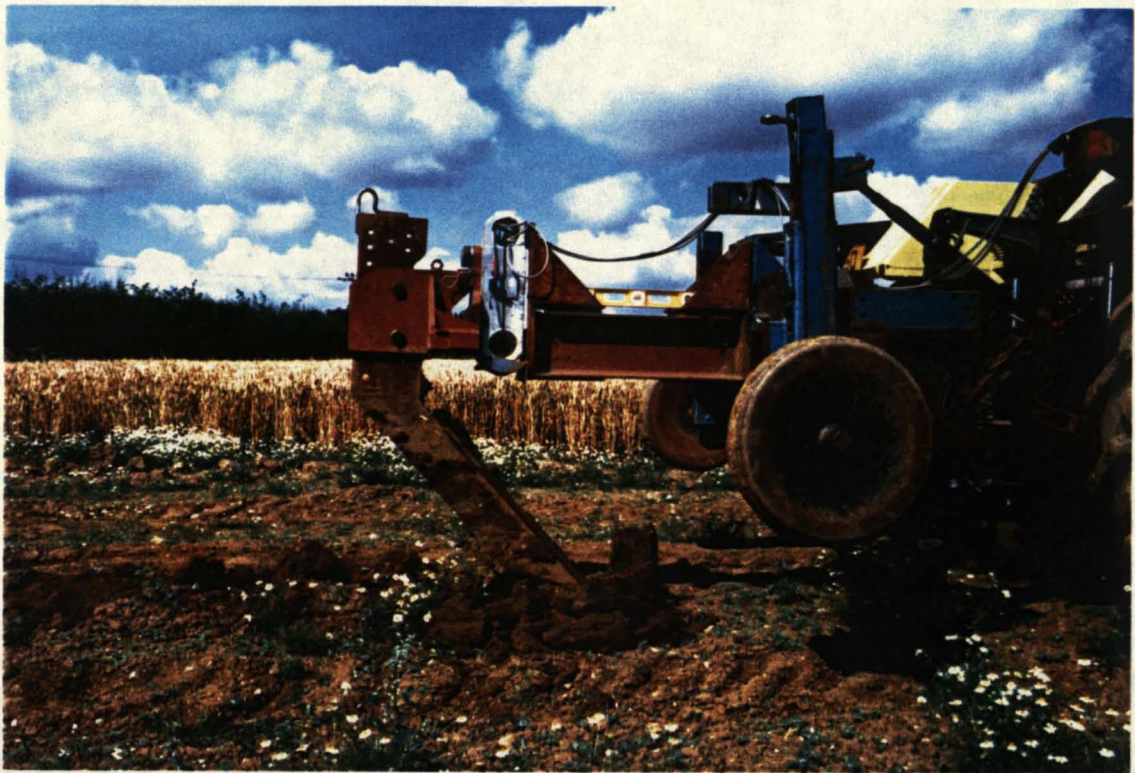
Plate 7. Extended Octagonal Ring Transducer between Tine and Frame
