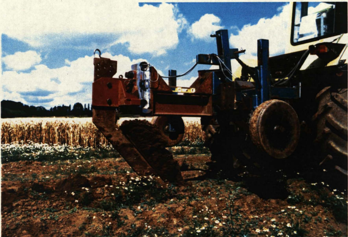
Plate 10. Standard Tine Hitched on to the Tractor
