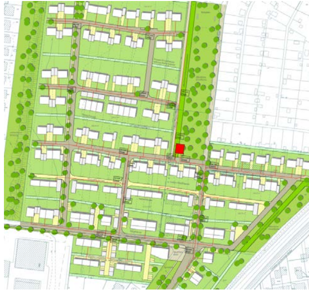
Figure 11. Map of investigated planning area “Zum Feldlager”; representation of the possible supply concept based on a district heating network with central heating plant (CHP plant) [20].
