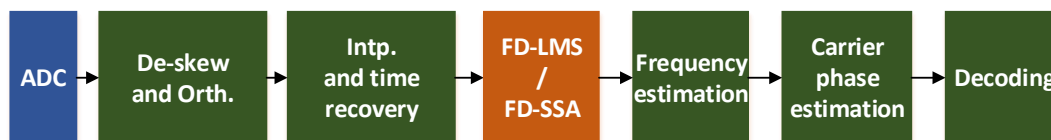
Figure 4. Full digital signal processing (DSP) stack of the single- and multi-mode DSP. Orth: orthonormalization, Intp: Interpolation.
