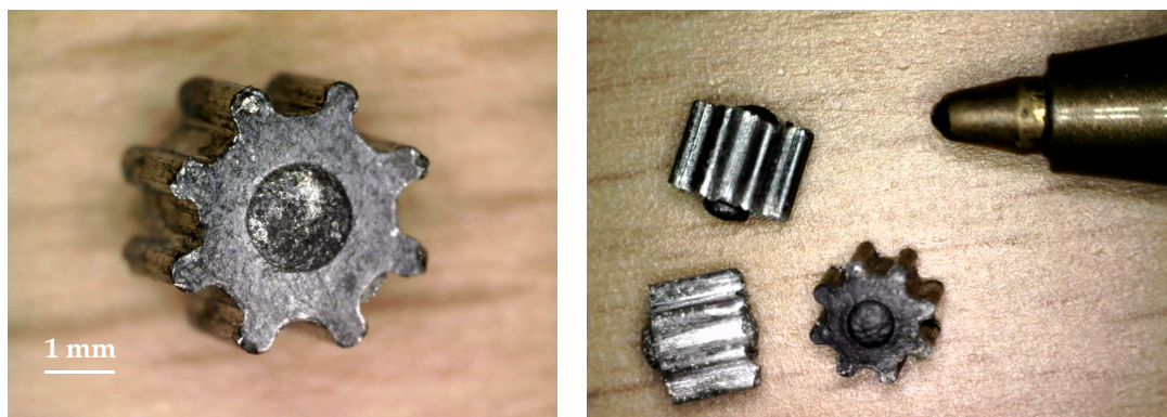
Figure 6. Examples of sintered samples using different process parameters. A pen tip was used to give an idea of the real size of the micro-gears.
