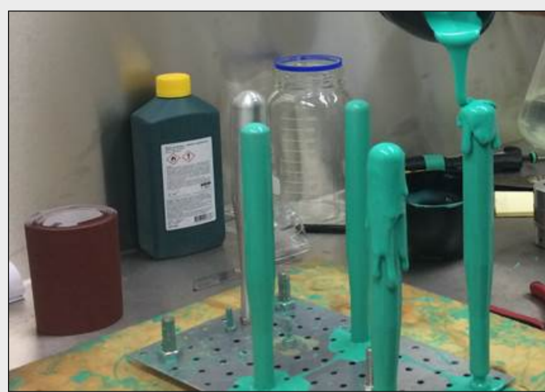
Fig. 2 Manufacturing of silicone core (on left) and a finished GFB (on right)
