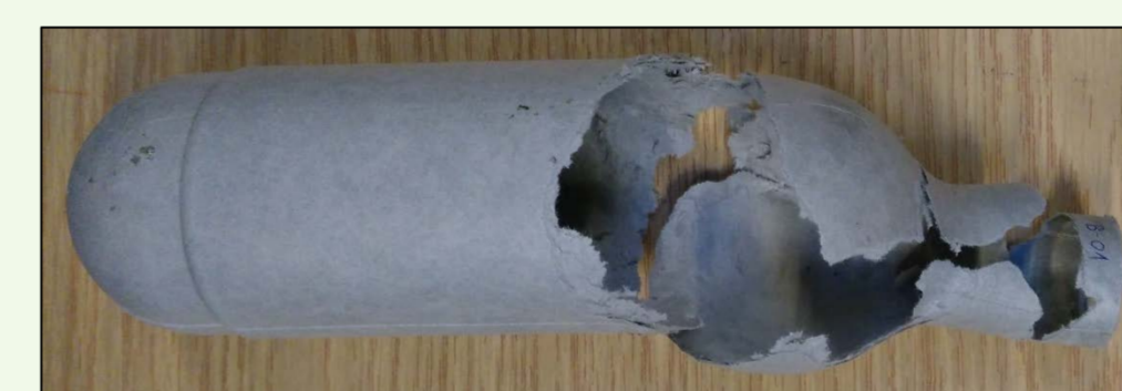
Fig. 5 Bursting of GFB (on left) and a prototype of GFB (on right)
