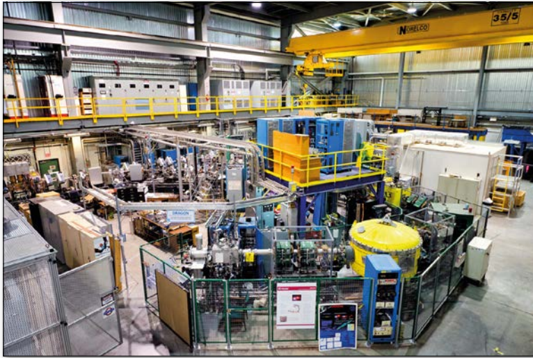
▲ FIG. 5: DRAGON, an example of recoil mass separator for the study of nuclear reactions of astrophysical interest, located in the ISAC facility at TRIUMF (Vancouver). Image courtesy of Steven Oates.
