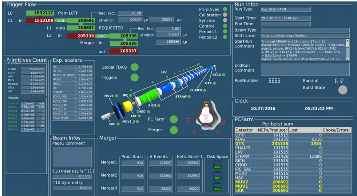
Figure 5.7: “Big Screen” of the Run Control displayed on a screen on the wall of the control room. It is the main tool reporting the status of the run, and allows quick detection of a problem in the data taking process.
