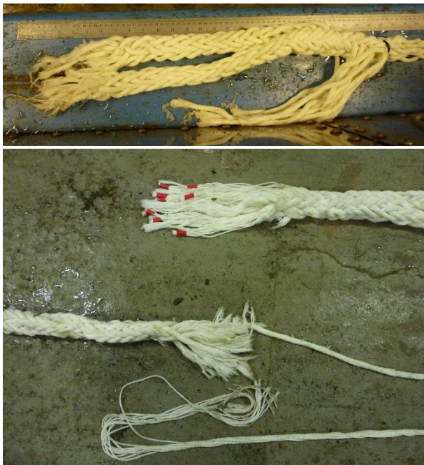
Figure 7: (top) PET and (bottom) PET-SSR samples after load-to-failure ISO 18692:2007(E) tests.
