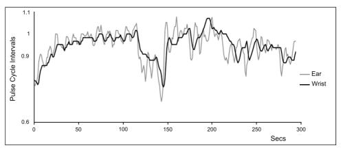
**Figure 2.** Pulse cycle interval data collected from the Mio Alpha 2 wristwatch (black line) and from the emWave2 ear sensor (grey line).
