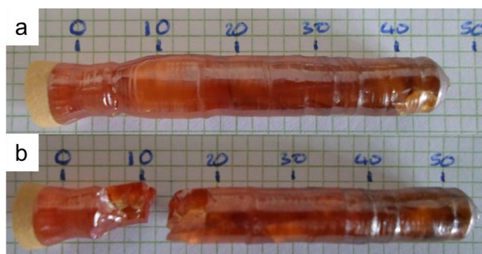
Figure 7.3: a) Image showing the entire length of the grown 42.5 mm \text{Bi}_{0.913}\text{V}_{0.087}\text{O}_{1.587} crystal rod; b) The fractured \text{Bi}_{0.913}\text{V}_{0.087}\text{O}_{1.587} crystal rod, showing the ~30 mm of crystalline material of the longest fragment.
