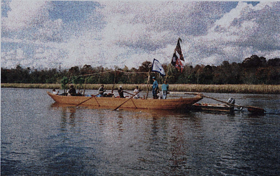
Figure 92: The Petersburg boat on the Savannah River. Note four rowing stations and sweep made from a natural bough (photo: Danielle Seward).
