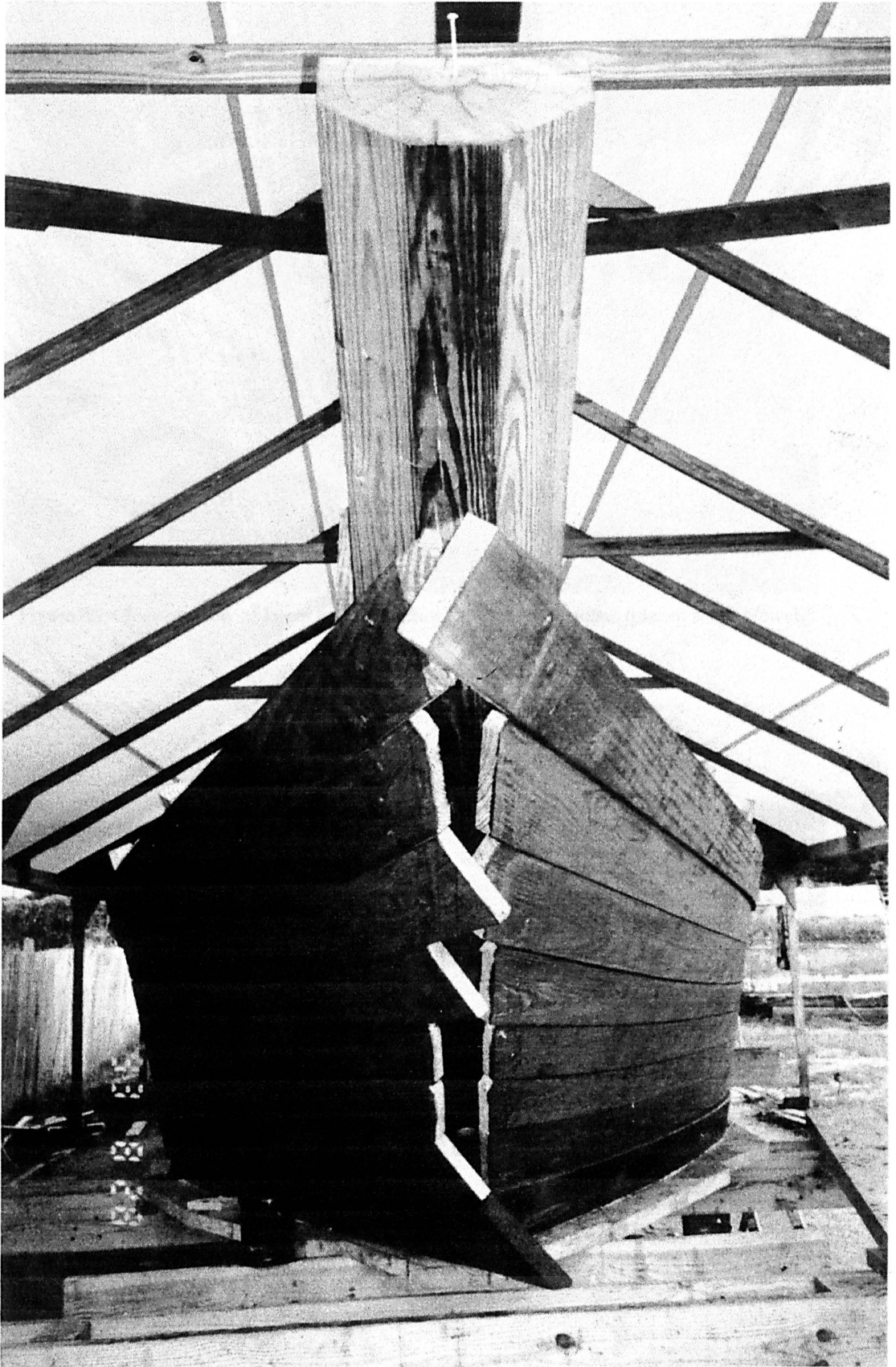
Figure 85: Untrimmed hood ends of the bow planking attached to stempost (photo: Mark Newell).
