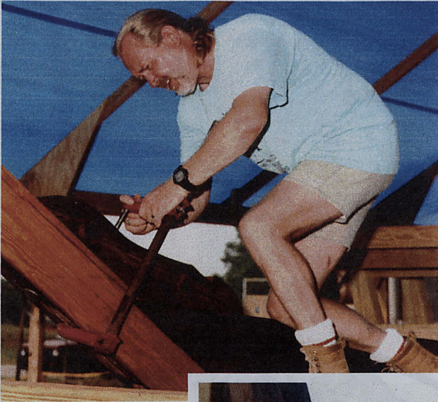
Figure 84: Above foregripe and stem knee assembly are unclamped by author after being bolted to stempost (photo: Danielle Seward) Insert - detail of assembly (photo: Mark Newell).
