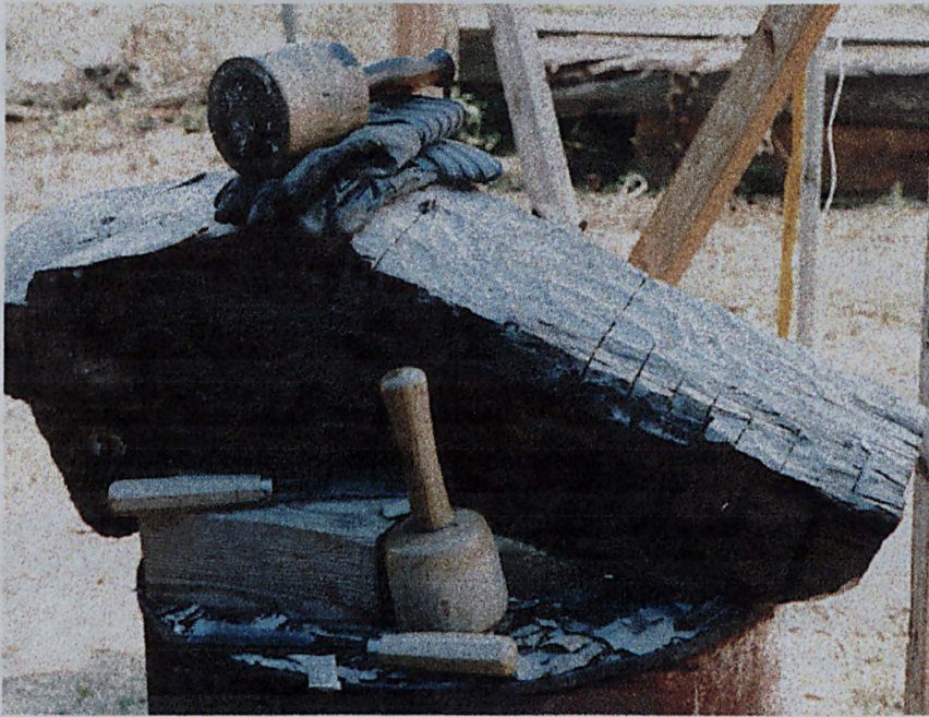
Figure 80: Partially carved stem knee for Petersburg Boat with author's tools used for the task (photo: Danielle Seward).
