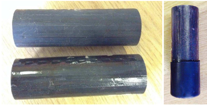
Fig. 5. Preparation of the corroding samples: original iron bar, bar coated with PCB lacquer, coated bar with set heat shrink tubing
