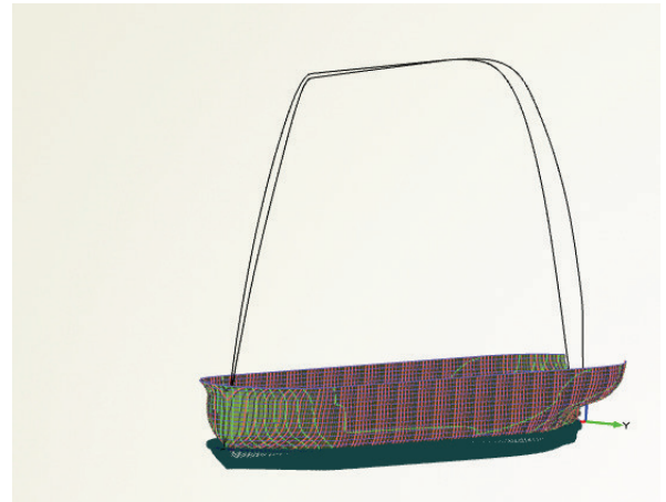
Picture 1: Finalized hullform after Lackenby variation
