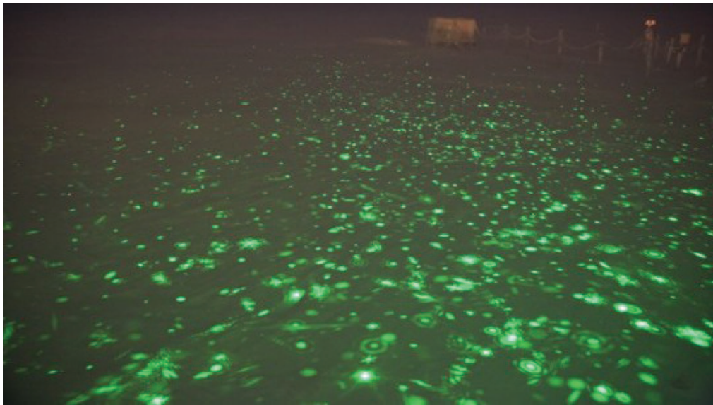
Fig. 1. Scattering from a lidar beam onto snow: 30 superimposed images, 1.3 s exposure time each. Recorded on 6 December 2016. The lidar hut is located behind and to the right of the camera, as shown in Fig. 2.
