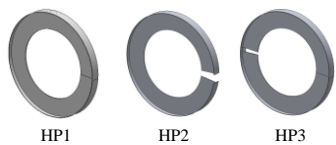
Fig.15 Solutions for reduction of eddy current loss
