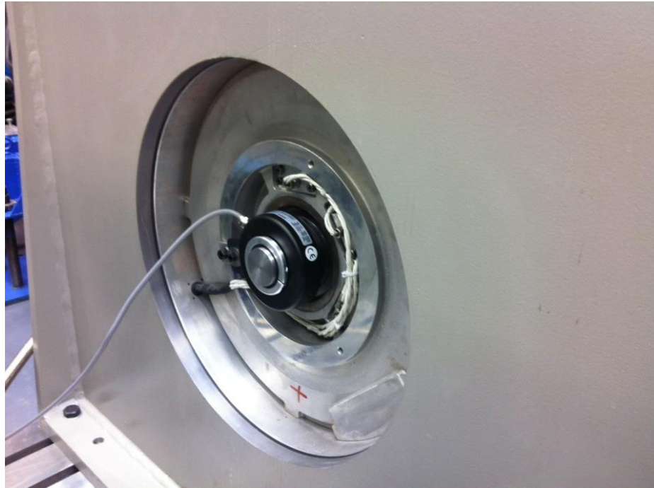
Figure 32: Encoder mounted on rear of the test machine
