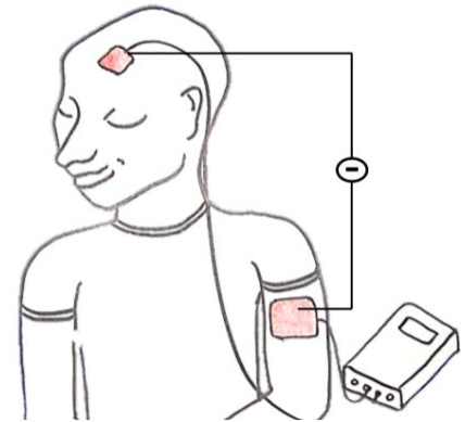
Figure 6.2. Schematic of electrode placement with the smaller electrode placed over the SMA, and the larger one placed over the upper deltoid muscle of the arm.
