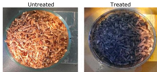
Figure 3-13: Heating heterogeneity in a single-mode cavity ( TM_{01n} ) (Robinson et al., 2015)
