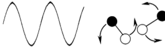
Figure 3-3: Dipolar molecules trying to align themselves according to the applied field (Lidström et al., 2001)
