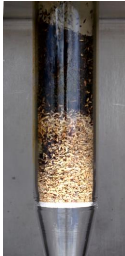
Figure 7-8: Non-fluidising pine particles leading to thermal runaway; particle size = 1.18-1.70 mm pine; initial mass = 70 g; gas velocity = 0.59 \text{ m}\cdot\text{s}^{-1} .
