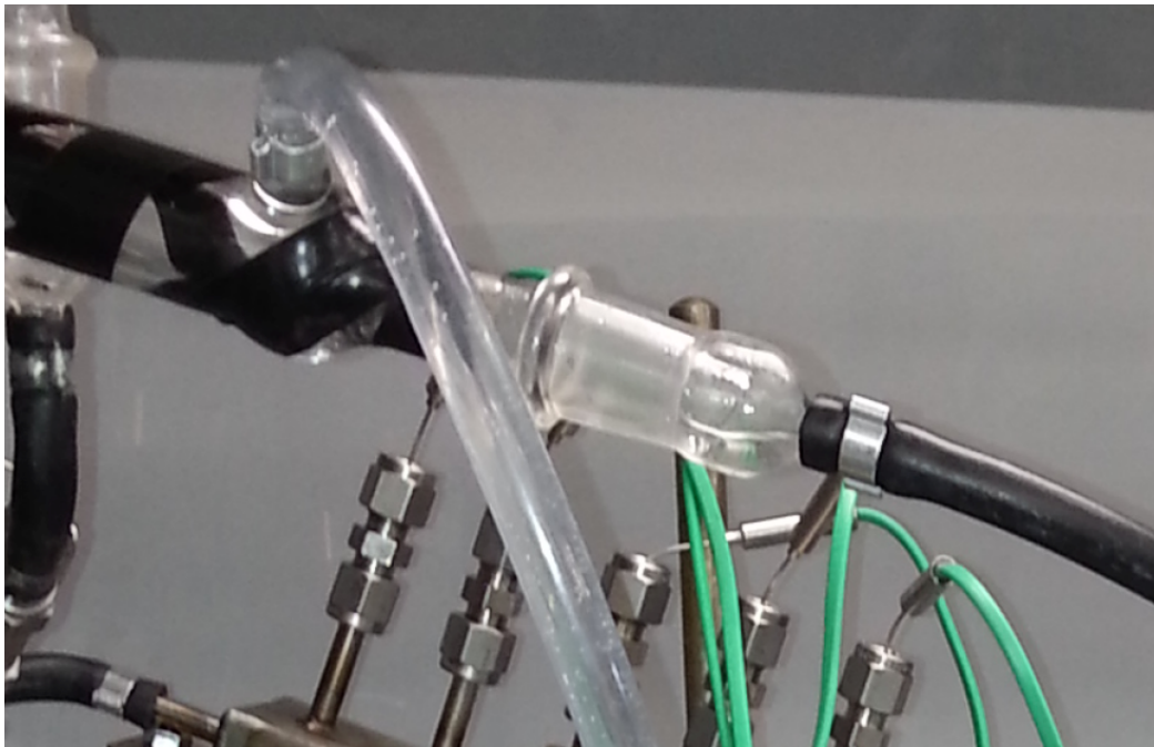
Figure 6.11: Photo of the condenser in the absorption refrigerator experimental test rig showing the refrigerant leaving the condenser as a liquid.
