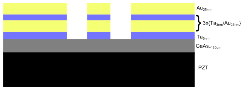
Fig. 3.22 Drawing of the multilayer structure used in the construction of waveguides. The waveguide is made up of Ta (blue) and gold (yellow). The waveguide is made with a 5nm base layer of tantalum on the surface of the GaAs (gray) followed by three identical bilayers of 25nm of gold followed by 3nm of tantalum. The whole structure is then capped with 25nm of gold. The GaAs is epoxied to the surface of the PZT piezoelectric transducer (black).
