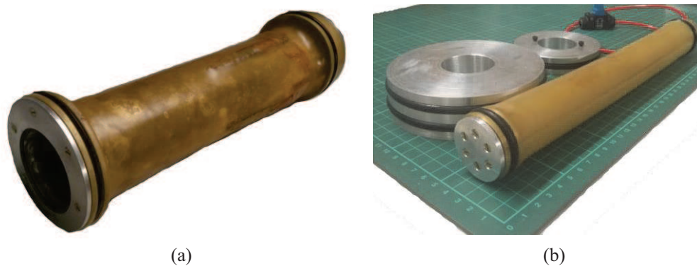
Fig. 3.2 (a) 90mm diameter model tunnel, (b) 40mm diameter model tunnel and its fitting rings.
