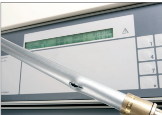
Fig. 3-5 Burst pressure test
