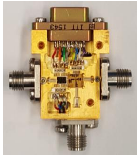
Fig.5. Photograph of packaged HTS receiver front-end module.
