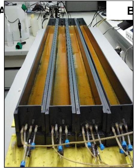
724 Figure 1. Schematic representation of the continuous flow bioreactor simulating natural 725 attenuation (A). The four channels fed with AMD and covered with the Fe-As biogenic precipitates at 726 the bottom (B).
