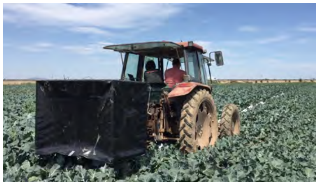
Figure 3: Set-up for data collection in Spain with the hardware platform mounted at the rear of the tractor.
