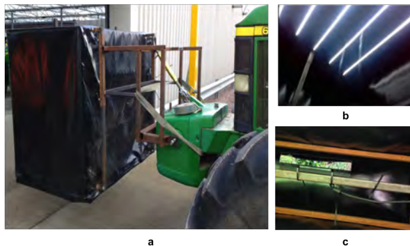
Figure 2: Enclosure and lighting set-up. (a) Manually adjustable shroud attached to the front of the tractor (b) artificial lighting using LED strip lights mounted inside the shroud to the top of the canopy (c) inside view of the enclosure with Kinect 2 mounted perpendicular to the field.
