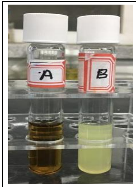
Figure. 6: Tube A showing visible colour change in reaction mixture of purified enzyme and \text{AgNO}_3 and tube B shows no colour change by inactivated enzyme and \text{AgNO}_3 .
