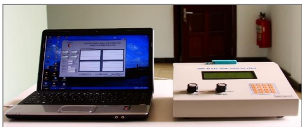
Fig.1 Portable and multichannel equipment for DNA virus detection developed by BIOMAT and NIHE.
