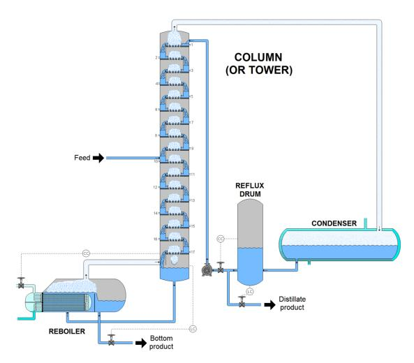
**Figure 1.1:** *Diagram of a distillation column. The mix from the reactor is fed into the column and then separated into two products. (Creative Commons by Marco Guzman.)*
