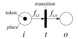
**Figure 3.5:** The simplest WorkFlow net with a single transition. Transitions represent tasks, places could be seen as conditions, and tokens are cases (e.g. a patient, a document or an image).
