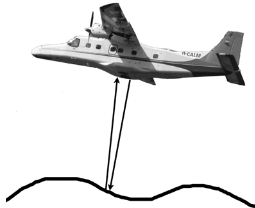
Figure 1.7 Basic principle of LiDAR operation. In addition to the laser sensor, onboard the aircraft (the Dornier 228 pictured here was used to collect data for this study) are GPS receivers and a gyroscope unit used to precisely measure the location and orientation of the aircraft.
