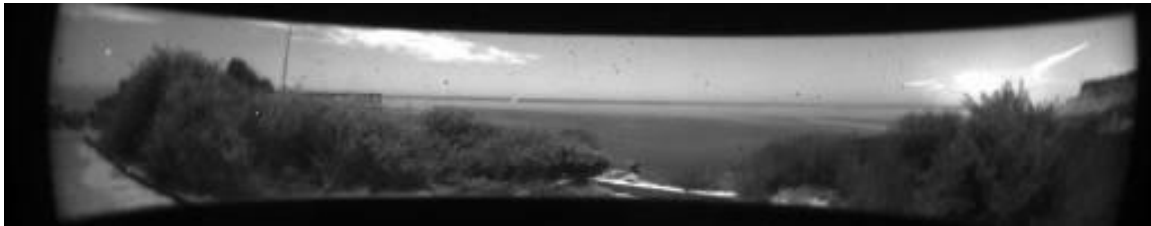
Fig. 10-3. Night Image near Full Moon: 4 Feb 2012 0600Z, Moon phase = .837, Open Hole 3 min exposure with no neutral density filter. Scene is a factor of 800,000 darker than daytime image in Fig. 10-5.
