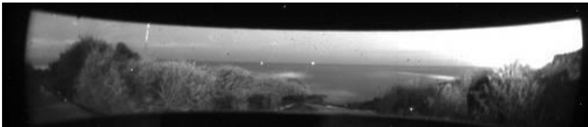
Fig. 10-4. Night Image under Starlight: 16 Feb 2012 0700Z, Moon 41° below horizon, Open Hole 10 min exposure with no neutral density filter. Scene is a factor of 4,000,000 darker than daytime image in Fig. 10-5.
