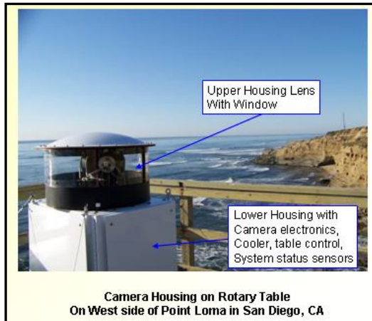
Fig. 6-4. MSI System on Pier
