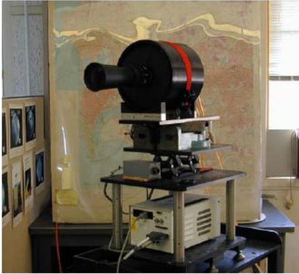
Figure A-2. MSI sensor head, with zoom lens and 16-bit digital CCD camera
