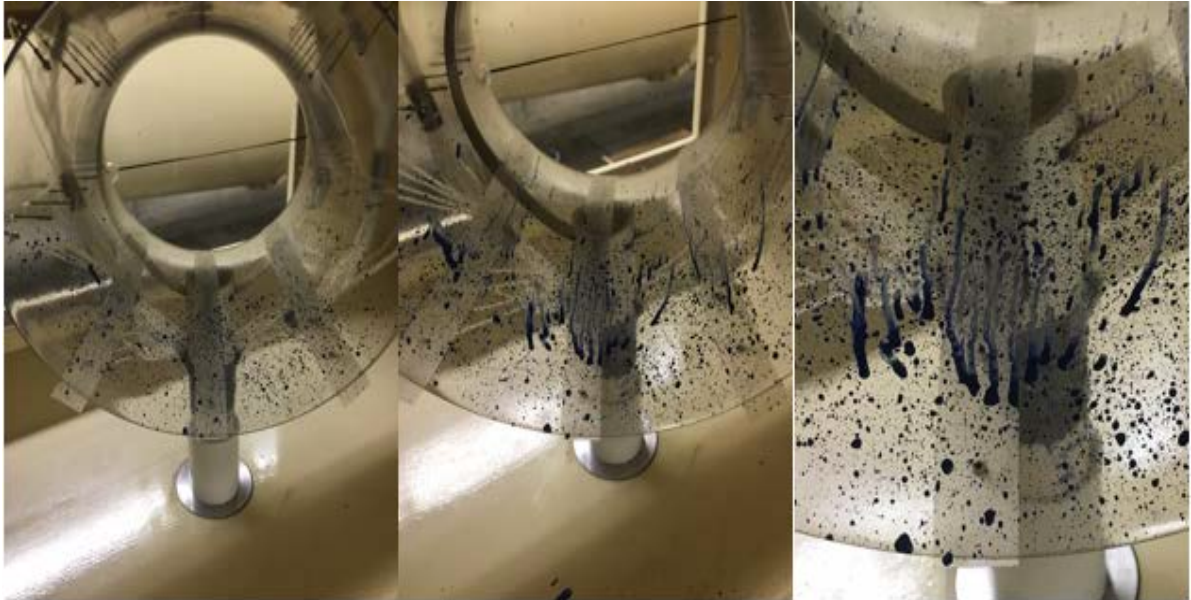
Figure 50. Model Three Oil Flow Visualization.
