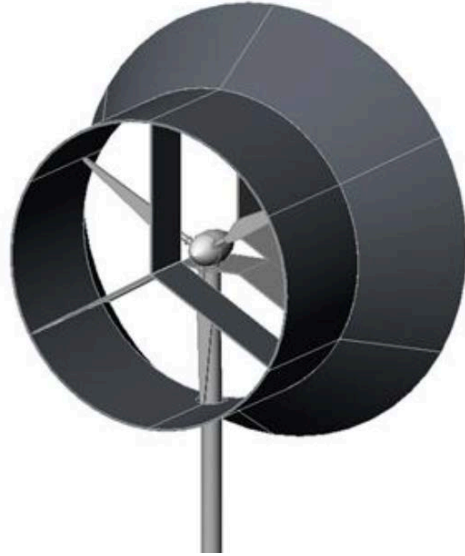
Figure 5. Wind Turbine with Shroud: Preliminary Design. Source: [8].
