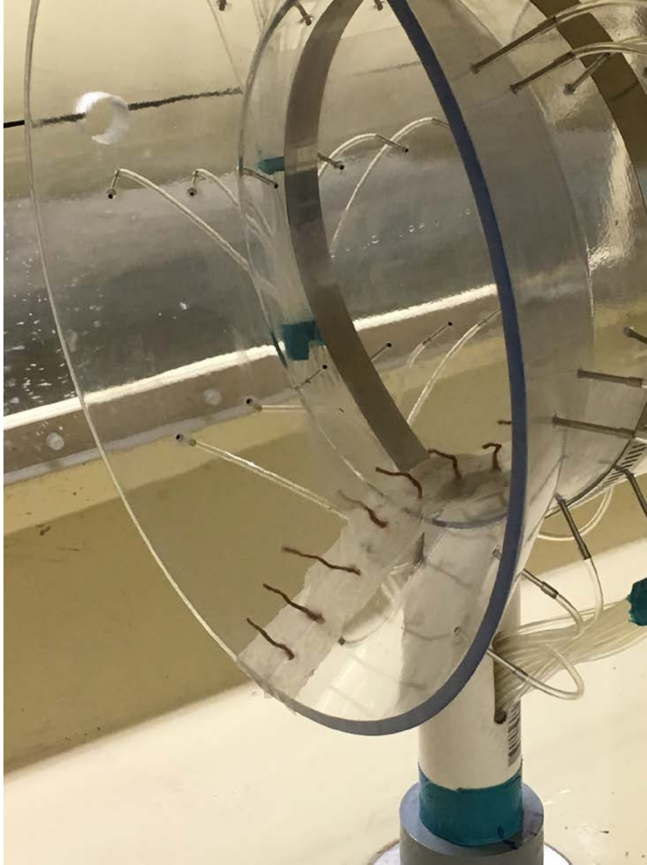
Figure 40. Model One Tuft Flow Visualization
