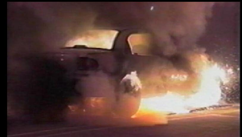
140 s: Gasoline-car interior alight. Tires later burst.
