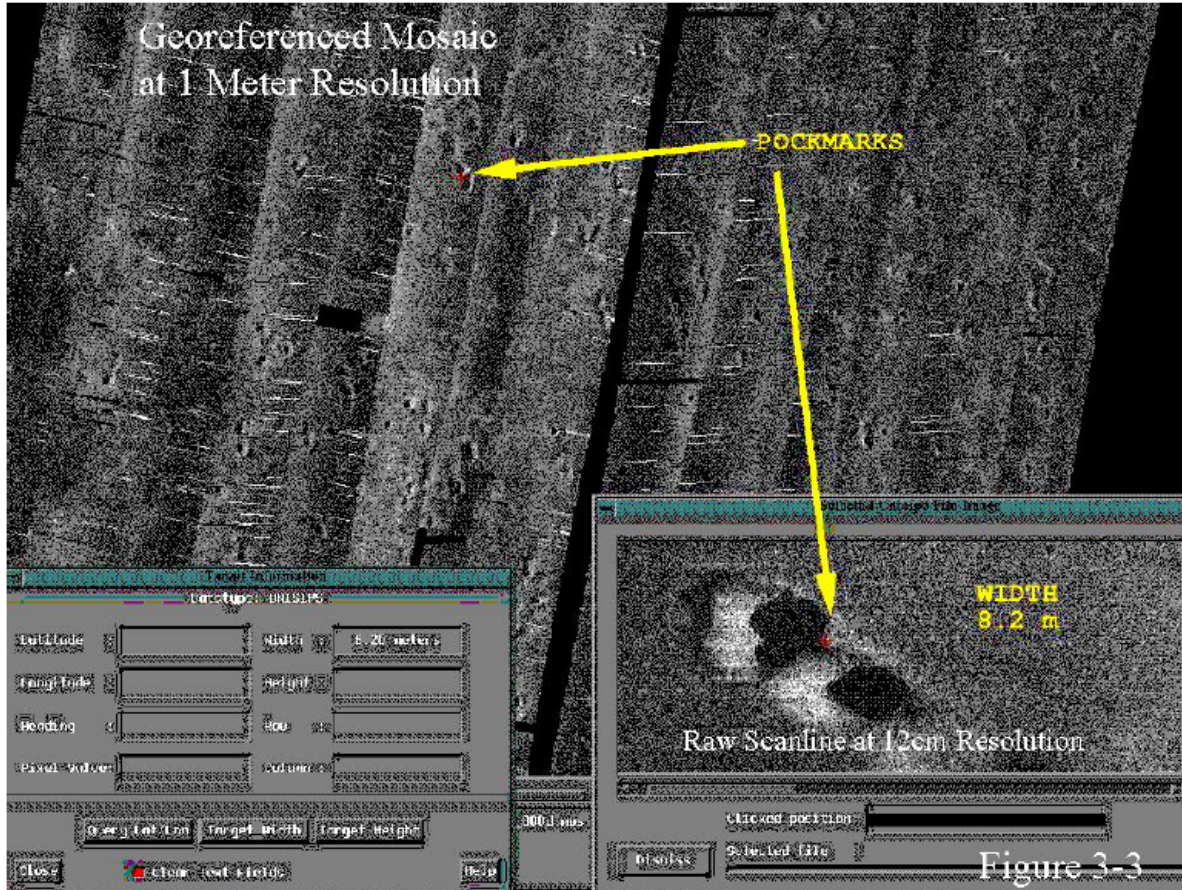
An acoustic imagery mosaic with one meter resolution. On this image numerous “pockmarks” can be seen. These features are likely to have resulted from seafloor release of hydrocarbon gases.
