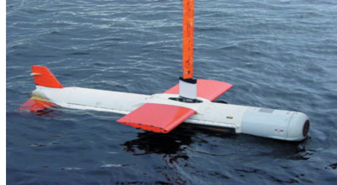
The Raytheon AN/AQS-20 Minehunting Sonar System, shown above, is the primary minehunting sensor system for the MH-60S helicopter, as well as the AN/WLD-1 Remote Minehunting System.
