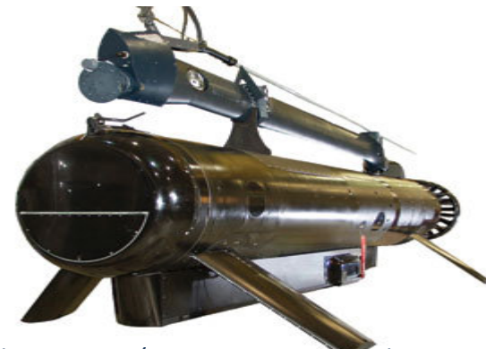
The Lockheed Martin AN/WLD-1 Remote Minehunting System is shown here with its snorkel folded for storage. The unmanned diesel submarine uses its snorkel for air intake and as an antenna mast while deployed in the ocean.
