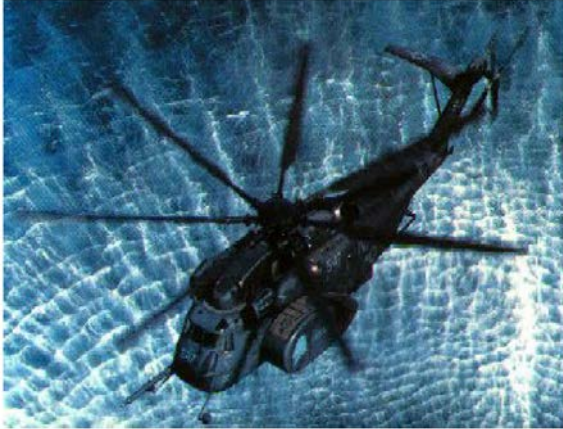
The MH-53E Sea Dragon class of helicopters have minehunting and sweeping capabilities using a variety of towed gear.
