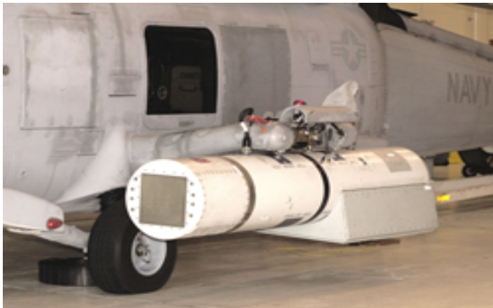
An early version of the Airborne Laser Mine Detection System. Northrop Grumman Photo
