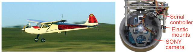
Fig. 1 Modified RC UAV with a gimballed camera and customized avionics.
