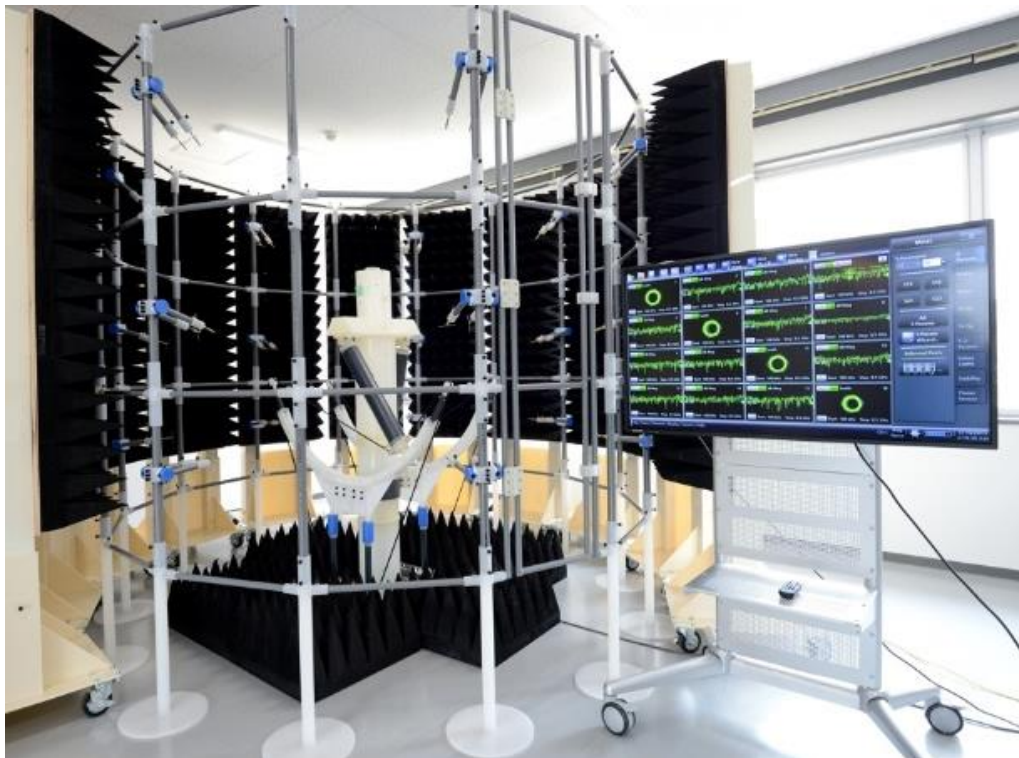
Fig. 5.17 Photograph of 3D-OTA apparatus with dynamic human phantom
