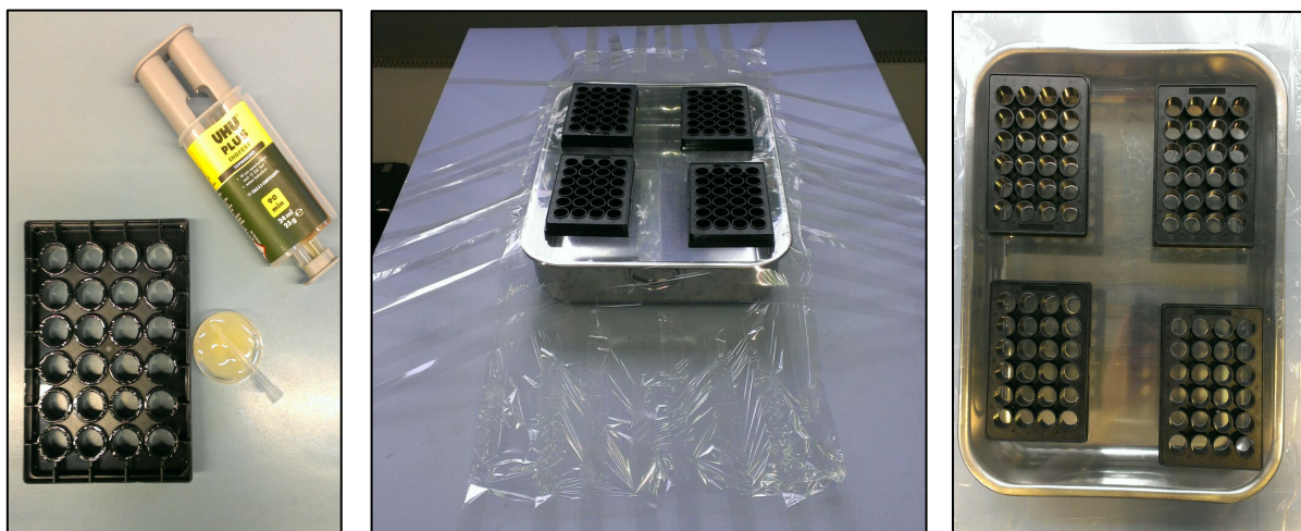
Figure 3.5 Preparation of 24-well plates with Mylar foil bottom. The bottom of each well was coated with epoxy 2-component glue and then placed on stretched-out Mylar foil to dry overnight.
