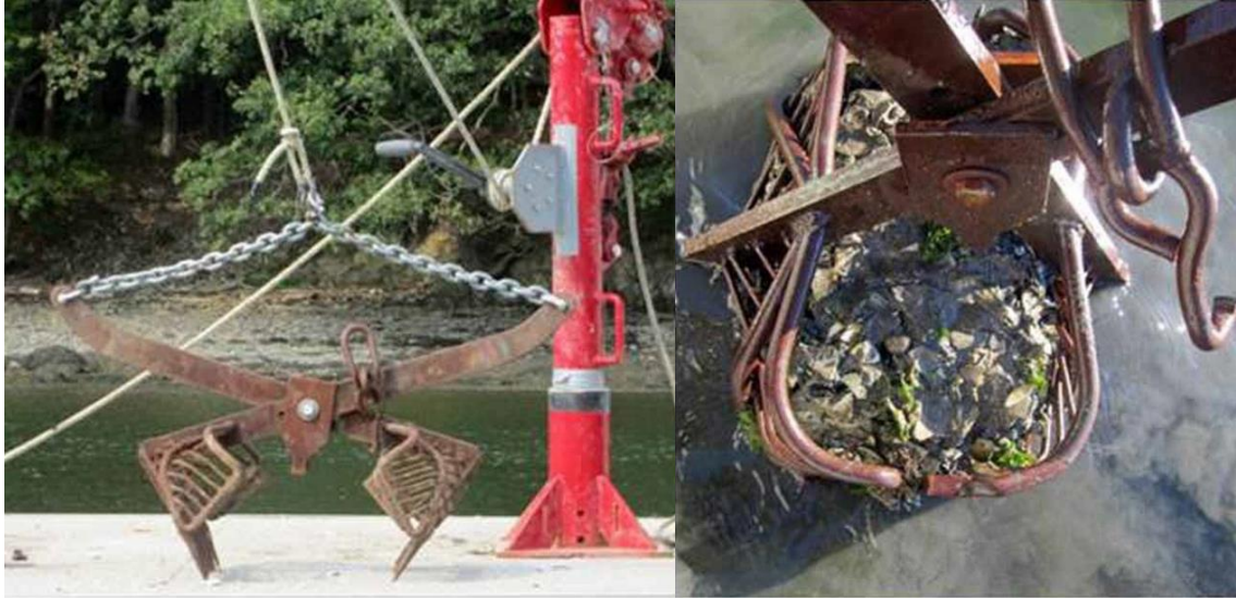
Figure 8. Patent tongs used to collect samples at native oyster reefs and restoration sites in 2013.
