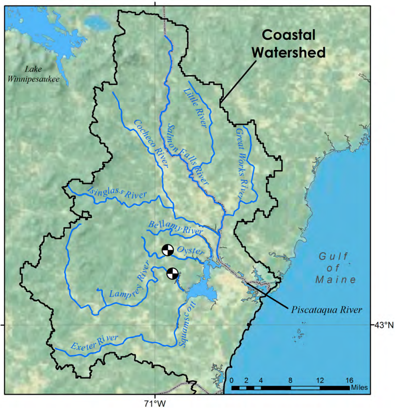
Figure 10. The Great Bay Watershed and major rivers that drain into the Bay. Long-term stream flow gages (black and white circles) have been collecting daily discharge data on the Lamprey and Oyster River since 1935.
