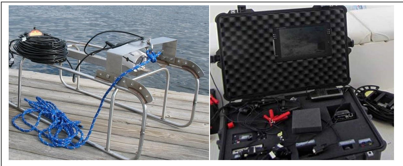
Fig. 4. Towed underwater video system (SeaViewer Model 650) used to determine reef shape, size and height. Left: camera mounted on sled. Right: imagery recorder and GPS unit.
