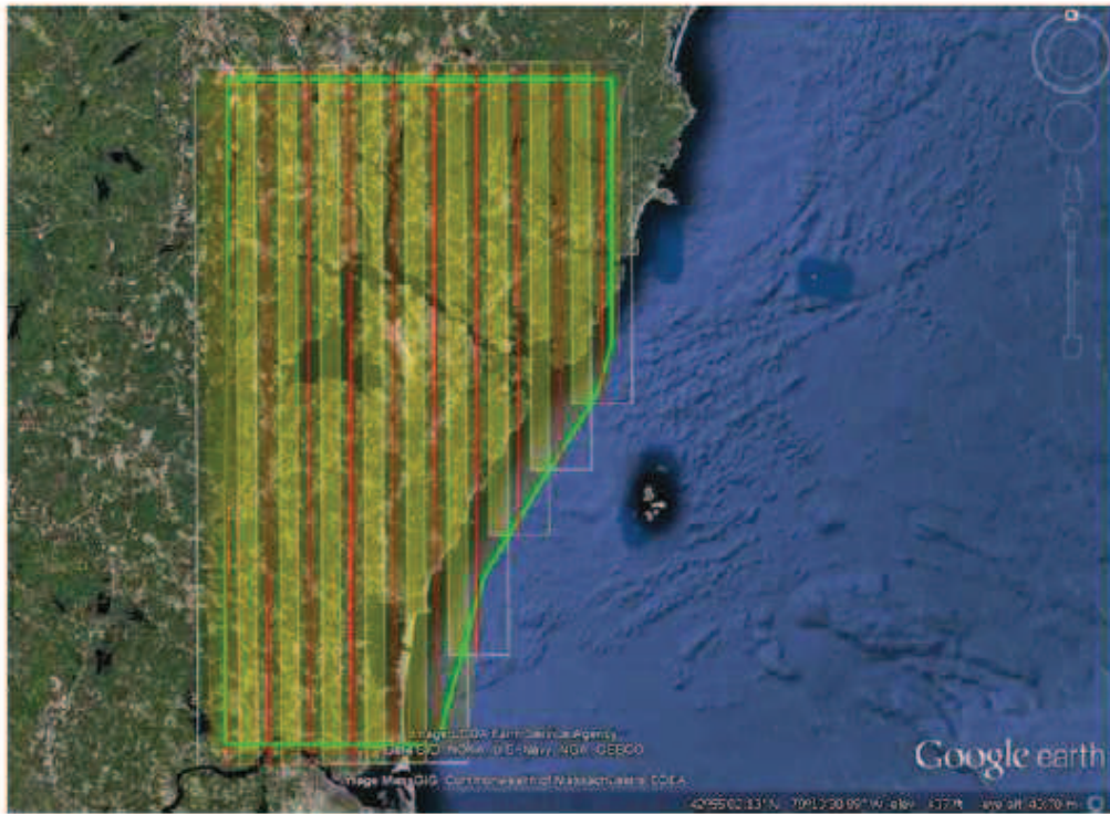
Figure 3: Flightlines for Aerial Survey (Reproduced from Appendix A, Figure 1). The green line is the project boundary, red lines are flight lines, and shaded areas indicate stereo coverage. Ground sample resolution for the raw imagery is 0.29 meters.
