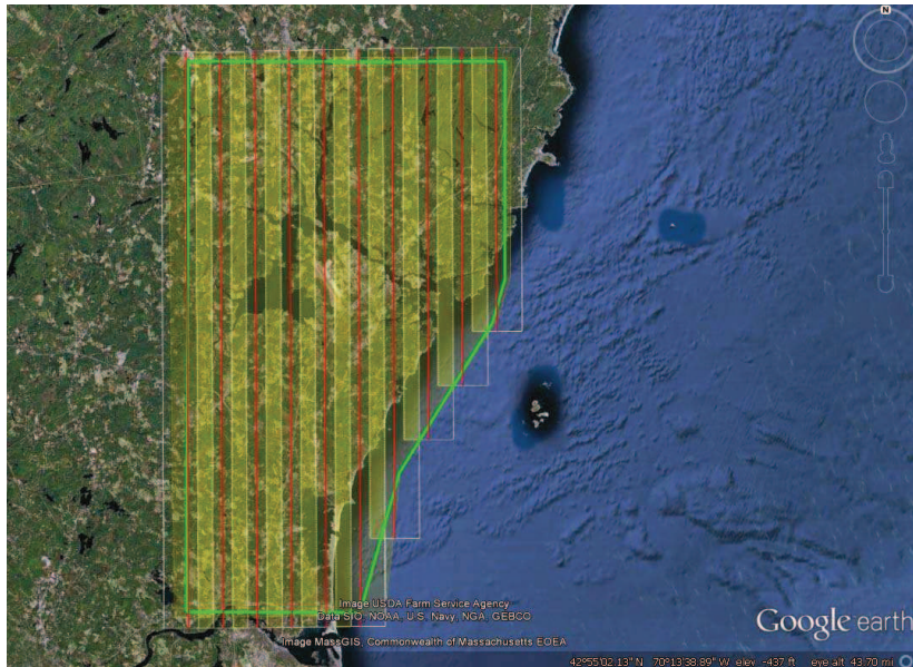
Figure 1. Flightplan layout consisting of 10 flightlines and 468 images. The green line is the project boundary, red lines are flight lines, and shaded areas indicate stereo coverage. Ground sample resolution for the raw imagery is 0.29 meters.
