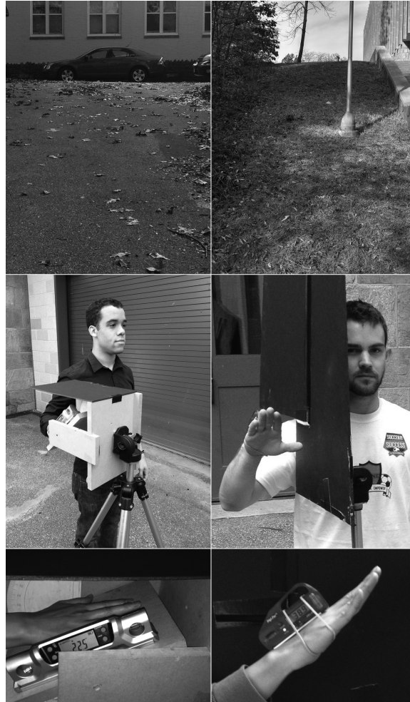
Figure 2. Hills used at SWAT (upper left; 6.3^\circ ) and at OSUM (upper right; 21.7^\circ ) are shown from the observers' viewpoint. Below are shown a palm board apparatus (middle left) with inclinometer (lower left) and a free hand apparatus (middle right) with inclinometer (lower right).
