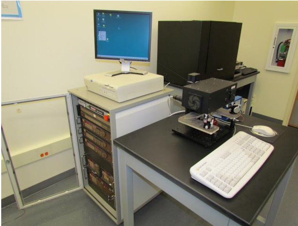
Figure 32. Current-Voltage measurement setup.
