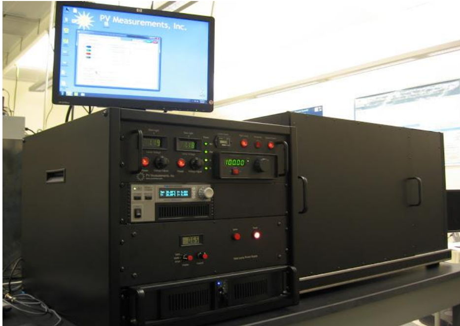
Figure 28. QEX10 Quantum Efficiency Measurement System, Inc.
