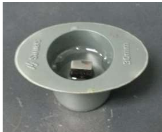
Figure 30 – Epoxy Hardening Container with Sample
