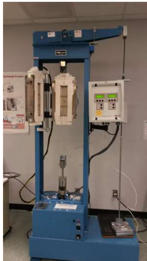
Figure 20 – Picture of the furnace being used for oxidation tests as part of the 2330 Series Creep/Stress Rupture Testing System
