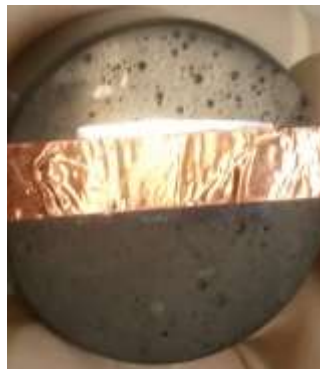
Figure 33 - C(T) Sample Prepared for SEM with Copper Conductive Tape
