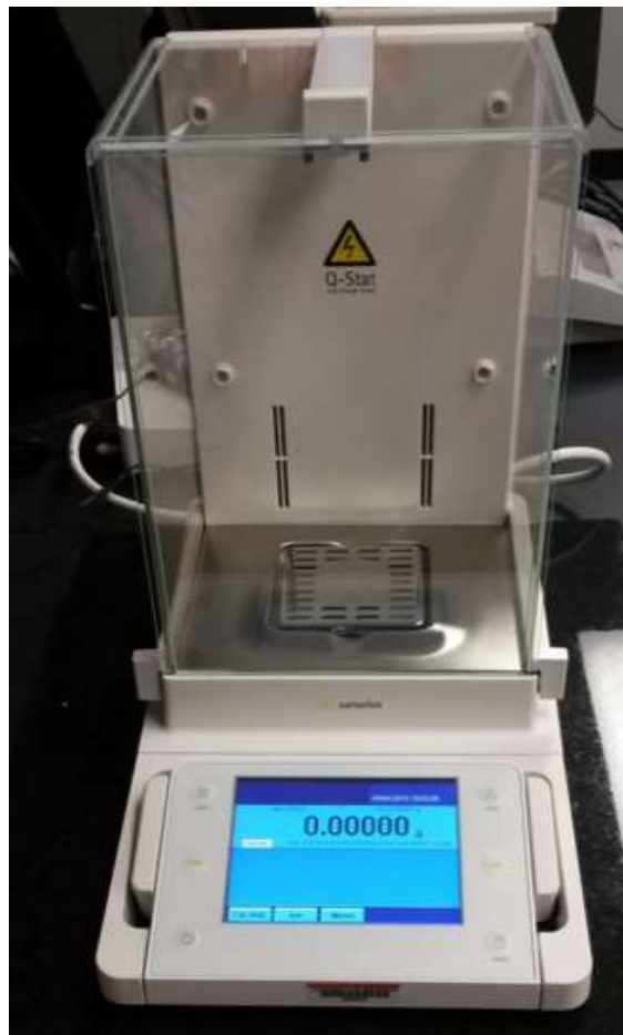
Figure 19 – Satorius Cubis MSA225S-100-DI used for Measuring Weight Change
