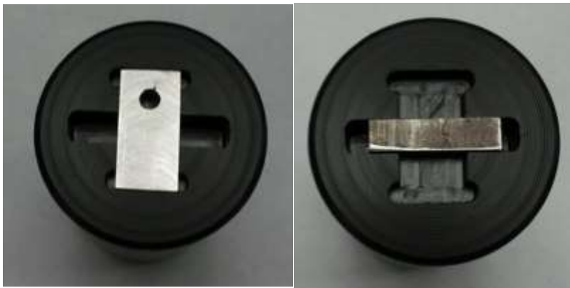
Figure 17 - A special sample holder created to ensure uniform polish on all surfaces
