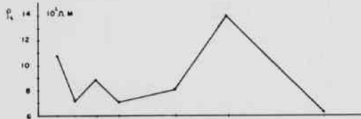
Figure 3B. Apparent resistivity of a Schlumberger profile with an electrode separation of 80 m.
