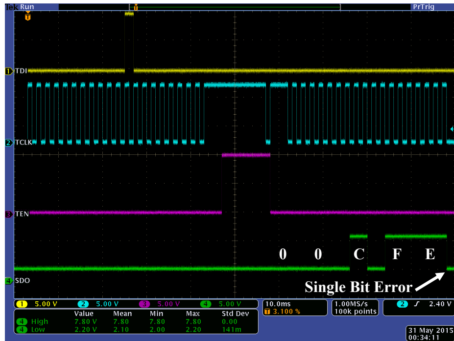
Fig. 6.18 R1C2 gate-drain Test with fault in 19 th bit. The yellow trace is the test data input (TDI), the cyan trace is the test clock (TCLK), and the magenta trace is the test enable input (TEN). The green trace observes the serial data output (SDO) from the gate driver IC. The serial data output reads 0x00CFE, which indicates a fault (expected 0x00CFF).
