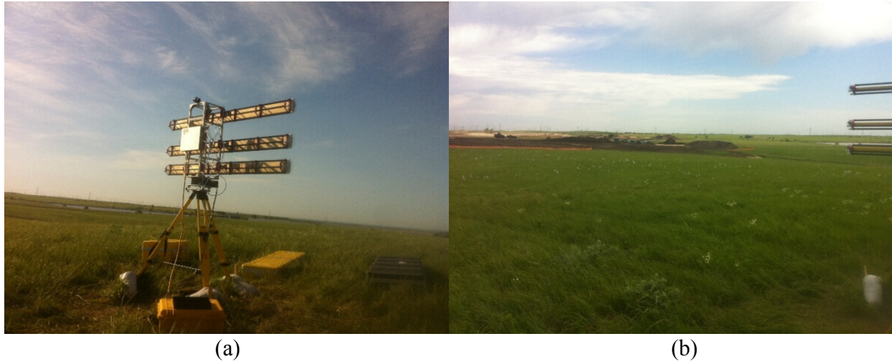
Figure 3.6. a) UMC GPRI-2 radar configuration as employed at the JEC project site showing instrument orientation, configuration, and anchor points, and b) view of the JEC project site from the overlook position showing relative site topography [images by author, in color].
