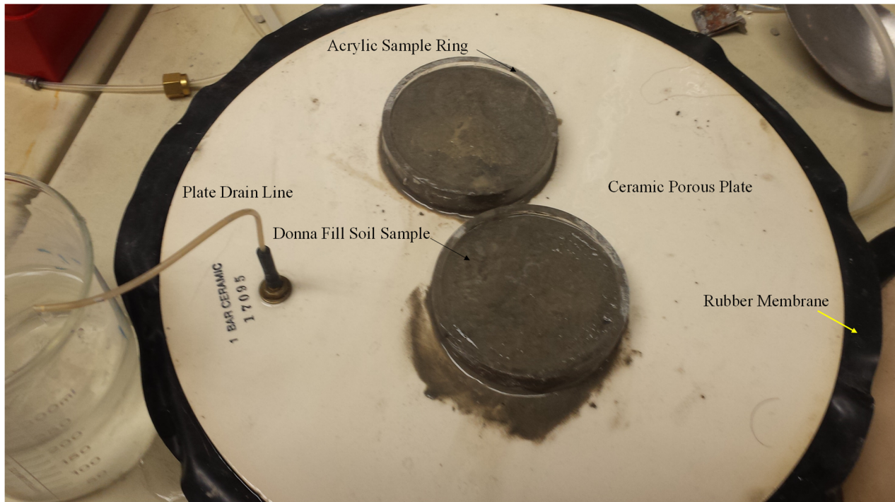
Figure 4.4. Porous plate for pressure plate extractor with two samples placed and extruded into sample rings for testing [image by author, in color].
