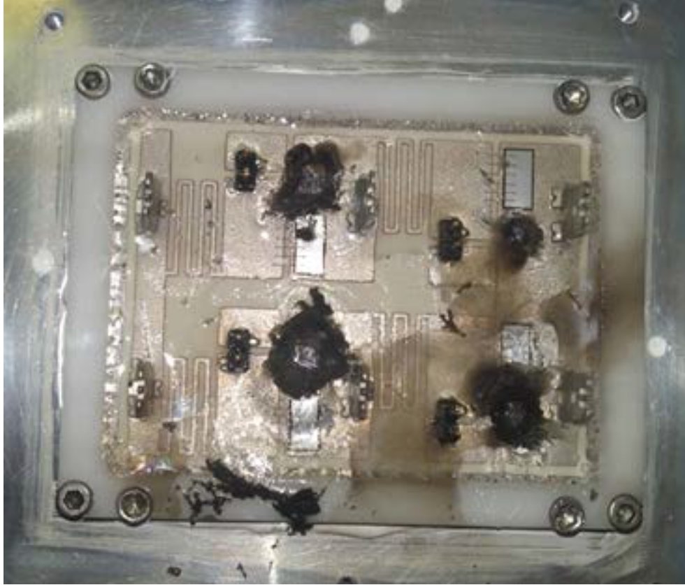
Figure 1: Catastrophic failure of an MCPM [1]
