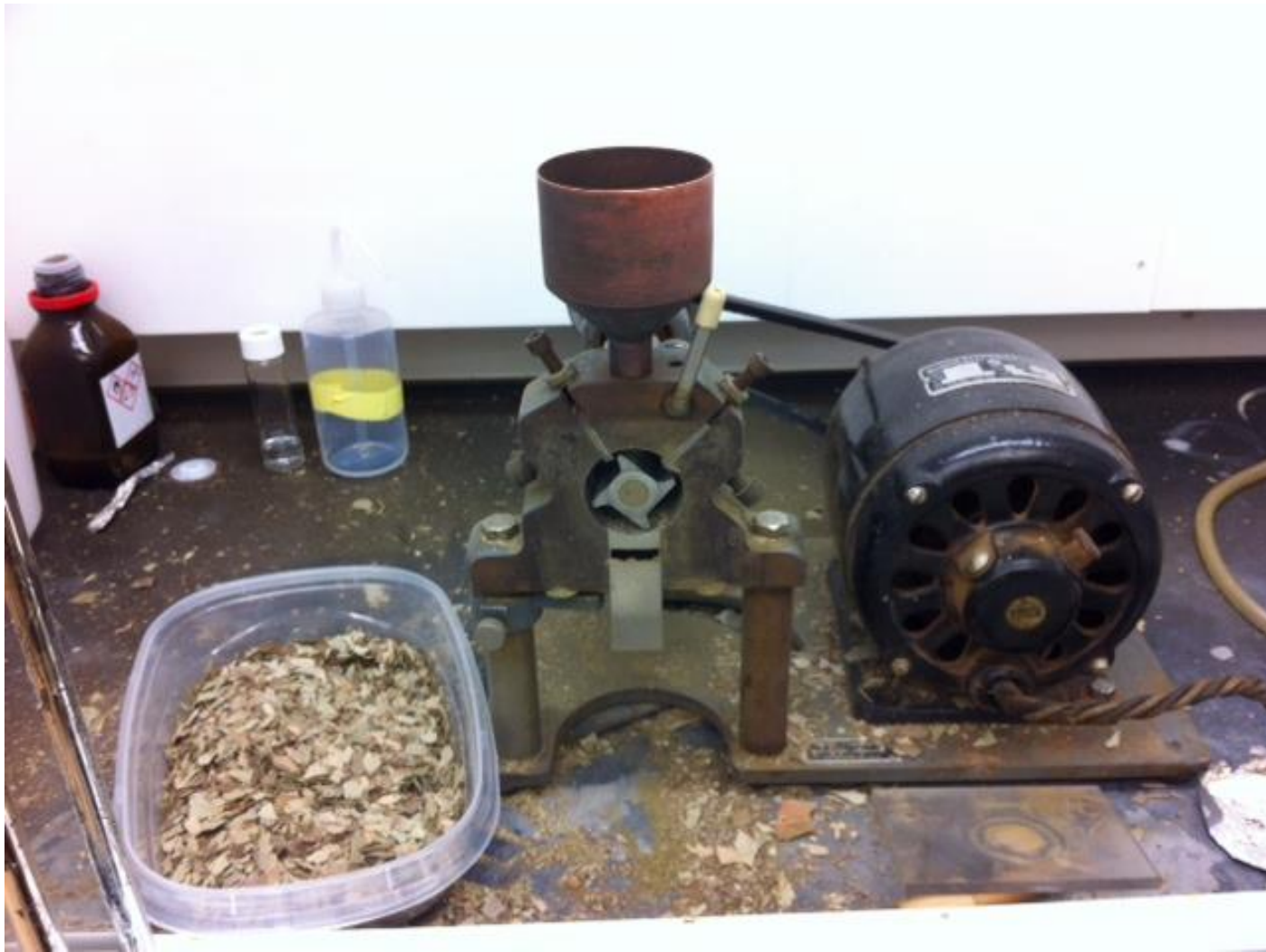
Figure 3.3. Image showing manually crushed leaves and the grinder used to finish grinding leaves to a fine consistency. The finely ground leaves were then mixed with potting soil for the allelopathy greenhouse experiment. Some of the leaves were also used in preparing aqueous solutions for the seed germination experiment (photo by the author).
