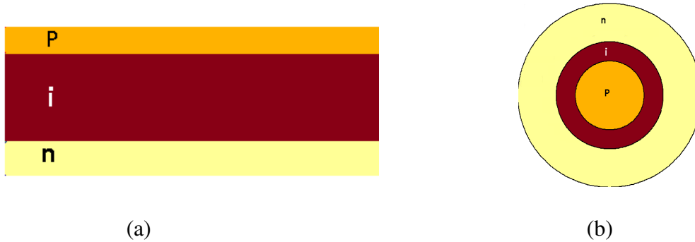
Fig. 6.7. Vertical cut plane to a flat PiN junction PVSC, and (b) Horizontal cut-plane of radial PiN PVSC
