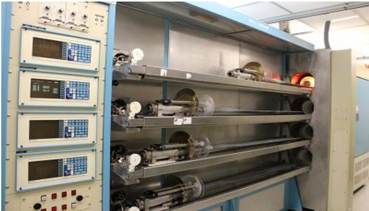
Figure 3.2: Four-stack oxidation/diffusion furnace consisting of a field oxidation, boron diffusion, phosphorous diffusion and hydrogen anneal (Bruce BDF4).
